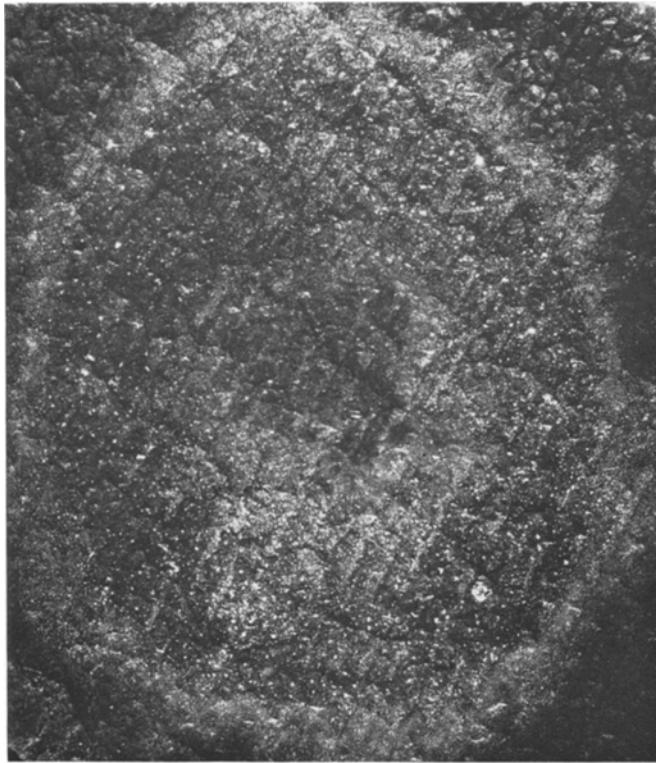
Fig. 1. Distribution of Ag salt on a pyrolytic graphite plate after heating a 1% \text{AgNO}_3 droplet at 300^\circ\text{C} in air for \frac{1}{2} h ( \times 10 ).
